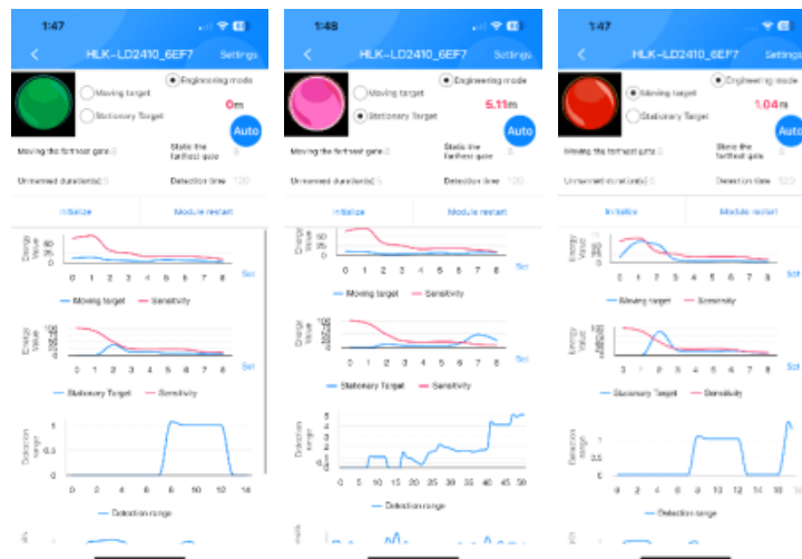
Figure 19. Controlling the device with the human presence sensor over the 5 m detection range
