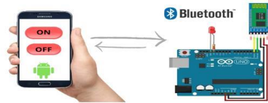
Figure 3. Bluetooth control app built with MIT App Inventor
