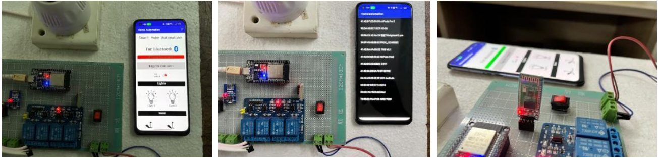
Figure 15. Connecting the custom app with the Bluetooth module
