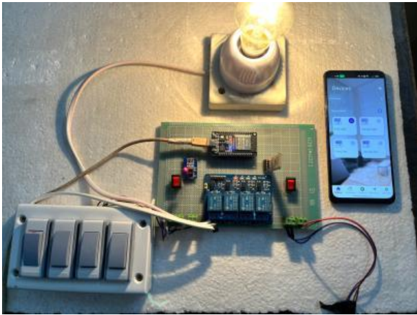
Figure 9. Controlling the device with the manual switch setup
